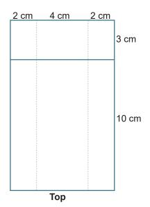
NOTE: the measurements on this diagram show the actual length that your lines should be (all real-life measurements divided by 10).
